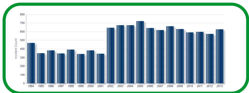
Figure 6 The number of US pipeline incidents (1994–2013) remains steady as more pipelines are laid.
