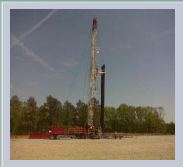
AFTER DRILLING **RIG RUNS AND CEMENTS CASING** IT MOVES OFF AND THE WELL **SERVICE RIG IS BROUGHT IN TO** FINISH THE WELL. THESE RIGS ALSO PERFORM MAINTENANCE **OPERATIONS ON WELLS**
