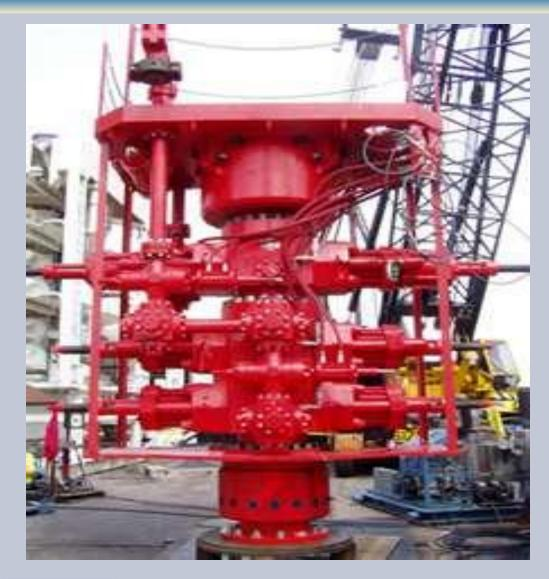
AFTER SURFACE CASING IS SET AND CEMENTED THE BLOWOUT PREVENT IS INSTALLED
