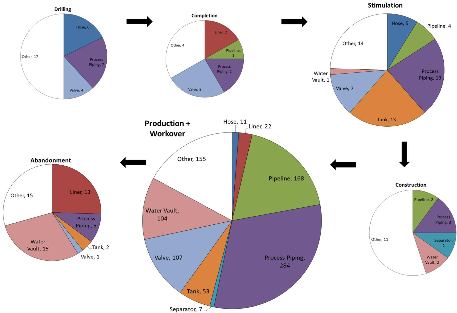
**Figure 4.** Equipment Failure by Operational Phase (counts)
