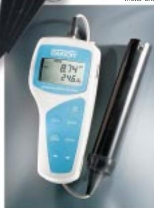
**One meter does it all—measure pH, conductivity and temperature without switching meters or probes!** Switch between conductivity and pH with a button press. Meters read pH from 0 to 14 pH, conductivity over four ranges up to 19.99 mS, and temperature in °C. Three-point pH calibration with auto-buffer recognition and four-point conductivity calibration provide high accuracy.
