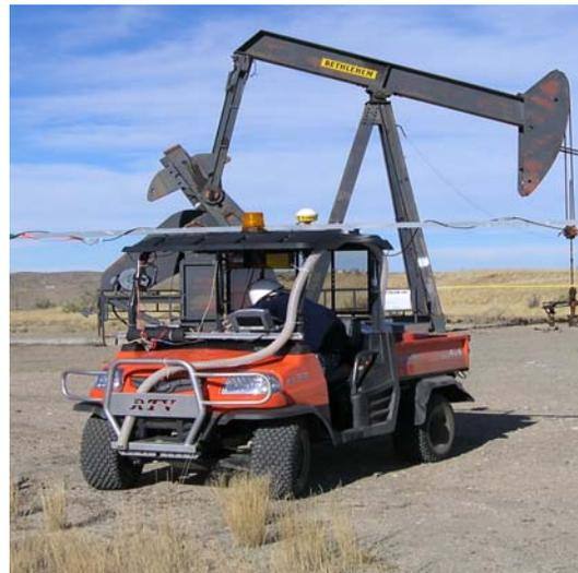
LDS is mounted on ATV and can be installed in truck, helicopter or other vehicle.
