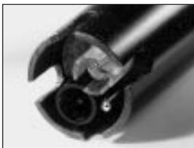
Easy-access 6-pin connector for probe is located on meter's top. Standard pH/CON 10 model also has connection for optional AC adapter.
