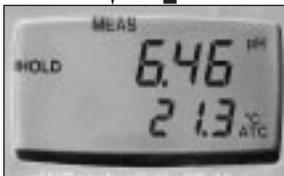
Multi-sensor probe features three different sensors, so you can take pH, conductivity, and temperature measurements with just one probe.
