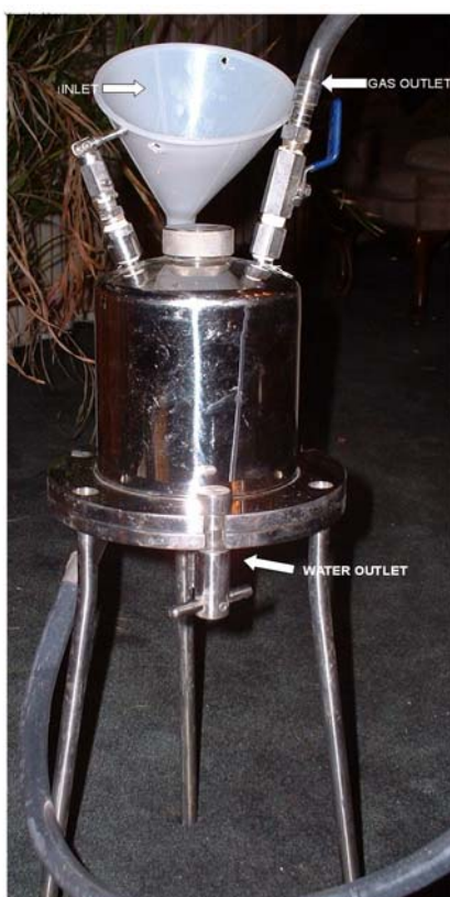
Figure 1. Sampling apparatus to collect methane gas in water samples in the Raton Basin.
