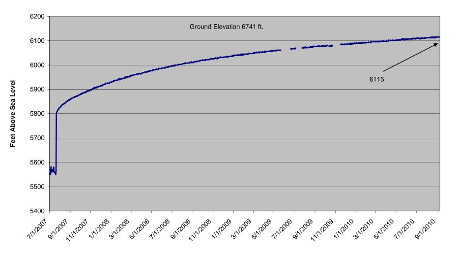
Rohr 08-01 CBM Well Static Water Level from 7/1/07 to 9/9/10 Well shut-in 7/20/07
