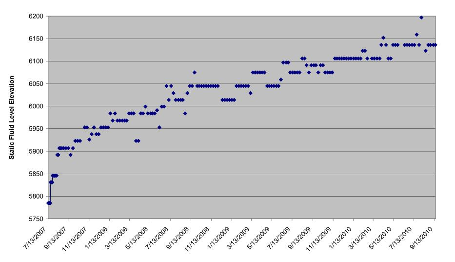
Rohr 04-14 CBM Well Static Water Level from 7/1/07 to 9/9/10 Well shut-in 7/20/07
