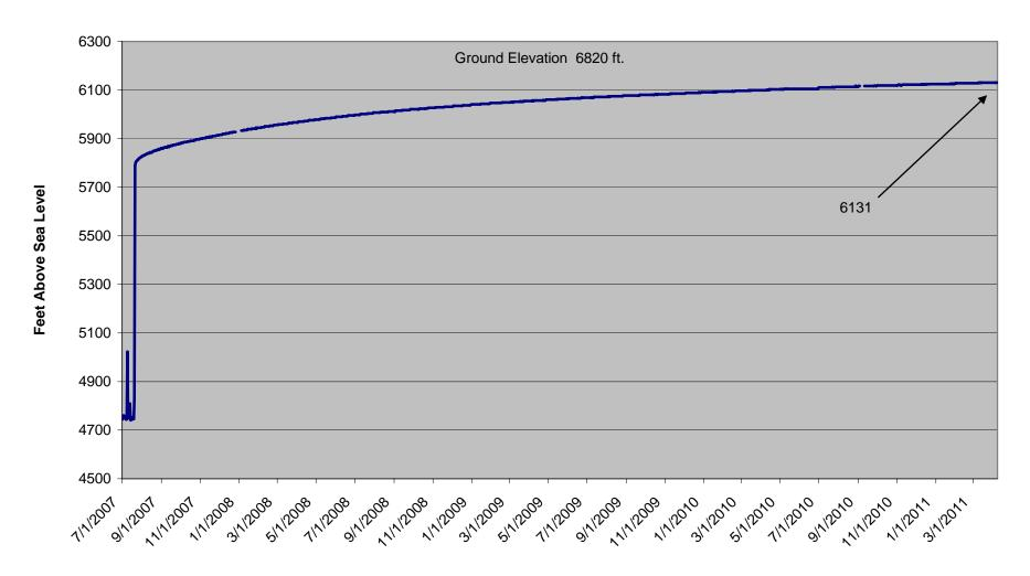
Rohr 09-04 CBM Well Static Water Level from 7/1/07 to 4/7/11 Well shut-in 7/20/07
