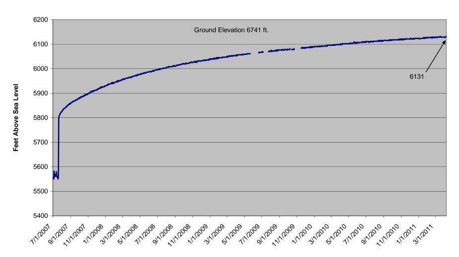
Rohr 08-01 CBM Well Static Water Level from 7/1/07 to 4/7/11 Well shut-in 7/20/07
