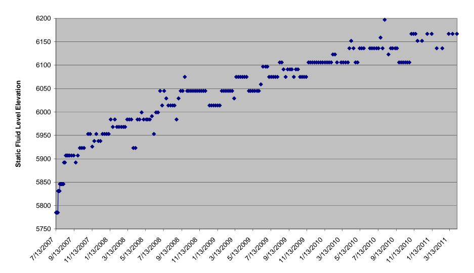
Rohr 04-14 CBM Well Static Water Level from 7/1/07 to 4/7/11 Well shut-in 7/20/07
