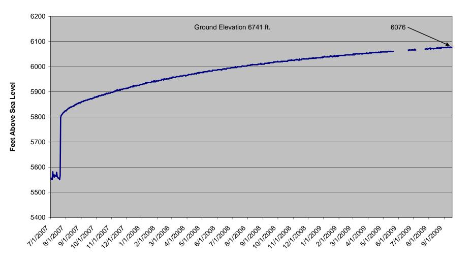
Rohr 08-01 CBM Well Static Water Level from 7/1/07 to 9/17/09 Well shut-in 7/20/07
