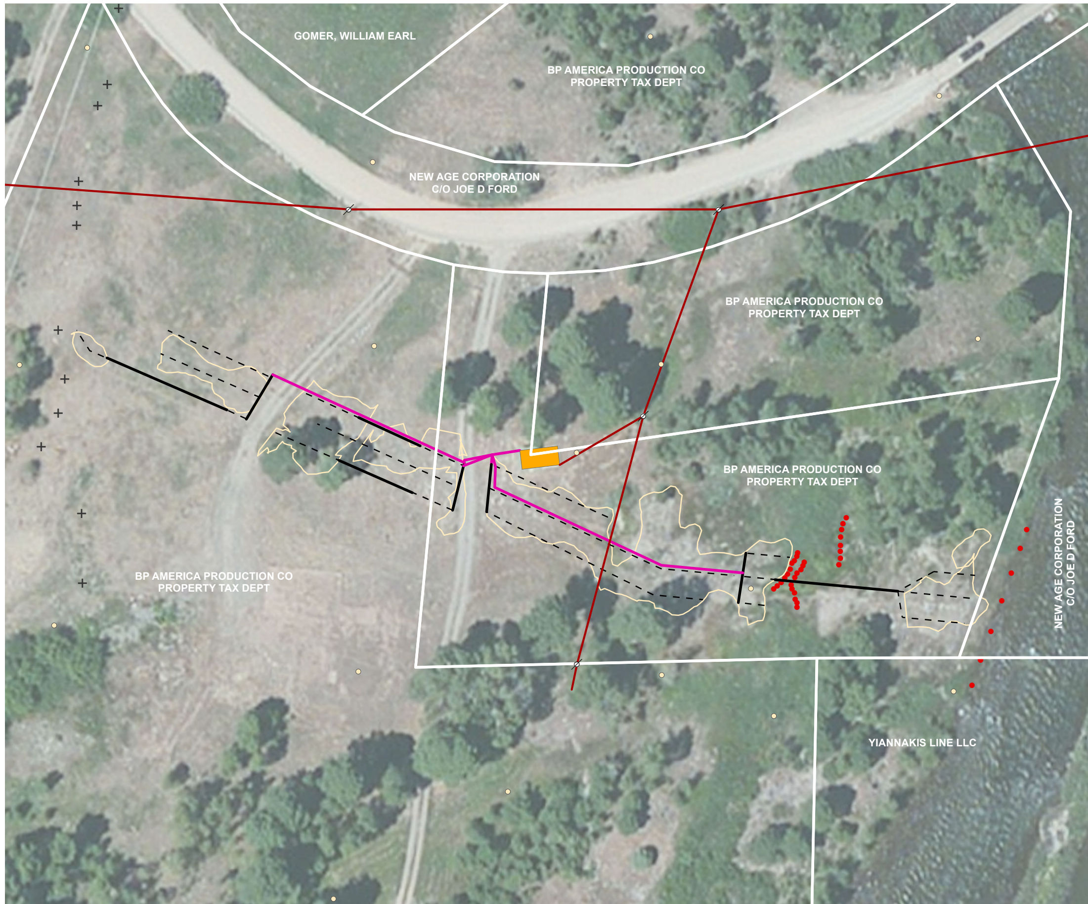
FIGURE 2 MITIGATION SYSTEM LAYOUT PINE RIVER 4M OUTCROP MITIGATION PROJECT DURANGO, COLORADO COLORADO OIL AND GAS CONSERVATION COMMISSION
