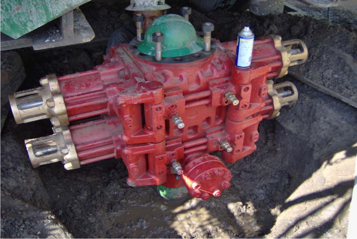
Photo 5: View of Blow-Out Preventer at the Wagon Gulch site.
