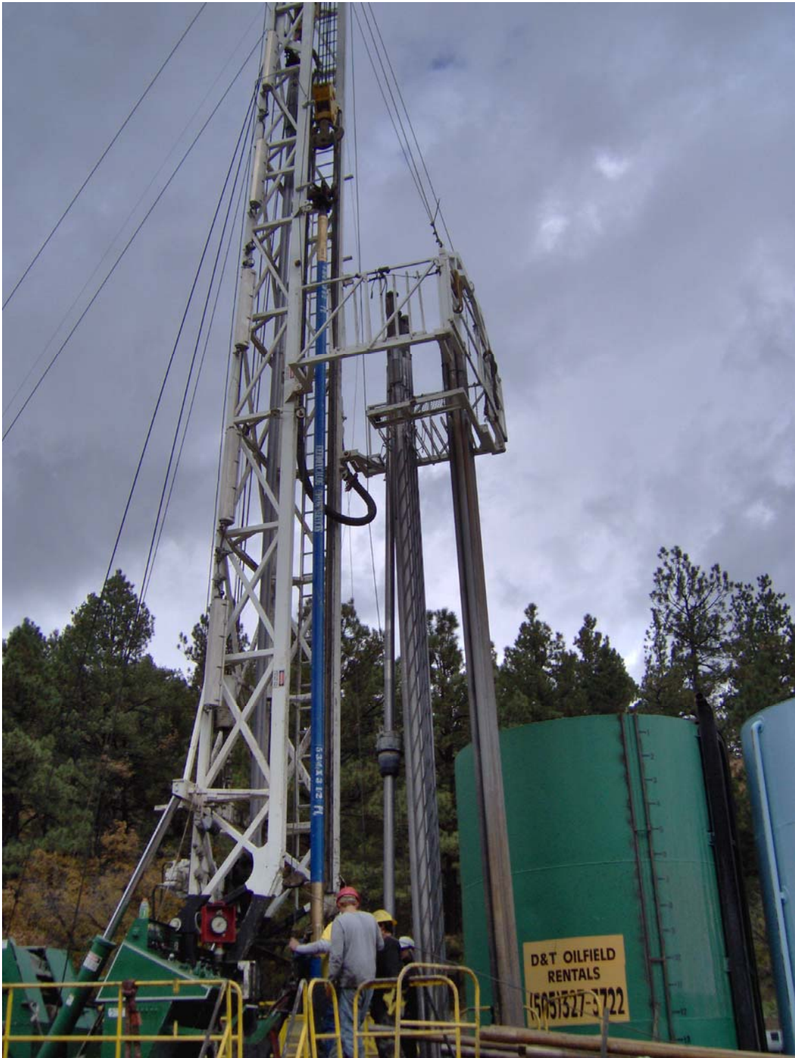
Photo 7: View of core barrel for coal core retrieval at the Wagon Gulch site.
