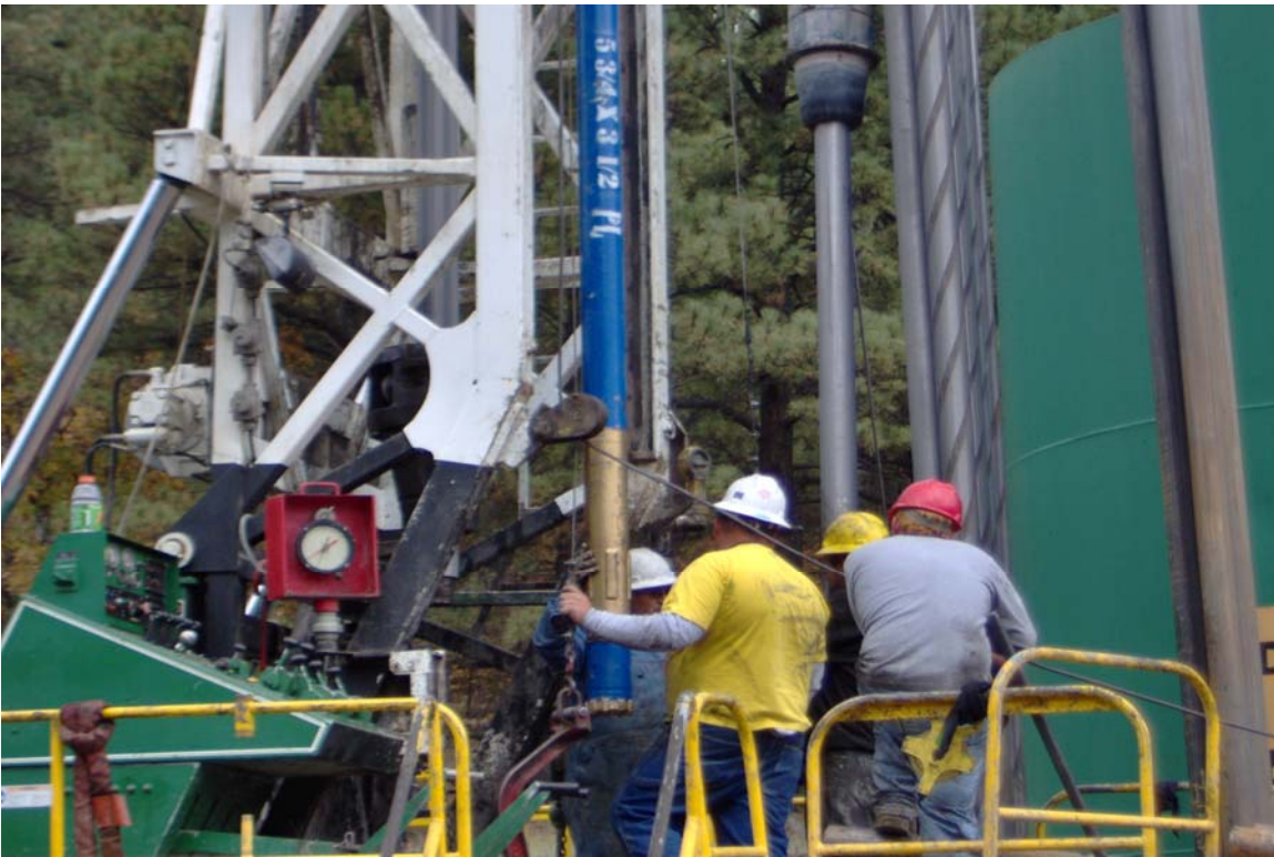
Photo 6: View of core barrel for coal core retrieval at the Wagon Gulch site.
