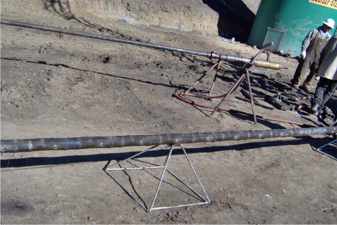
Photo 19: View of perforating tools at the Fosset Gulch site.
