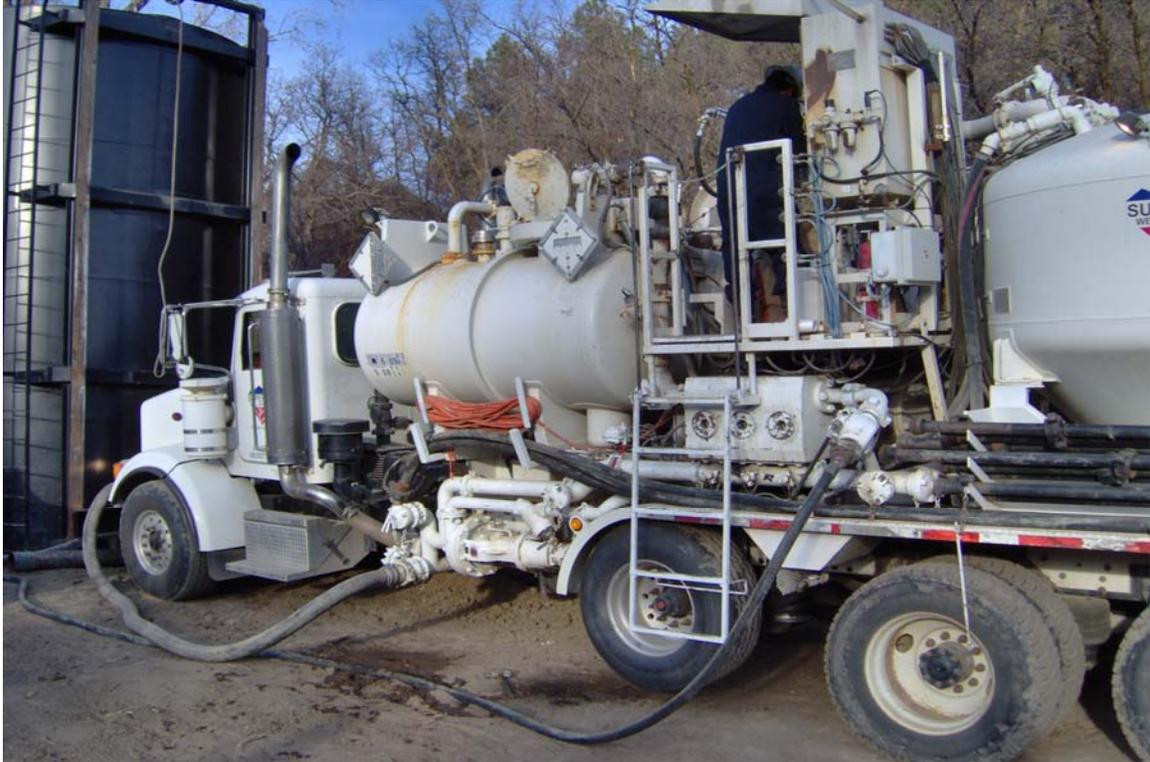
**Photo 21: View of cementing operations of the 4.5" casing at the Palmer site.**
