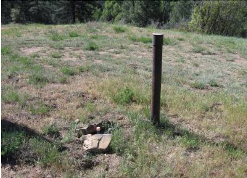
Schomburg #1 abandoned well marker and permanent gas monitoring probe.
