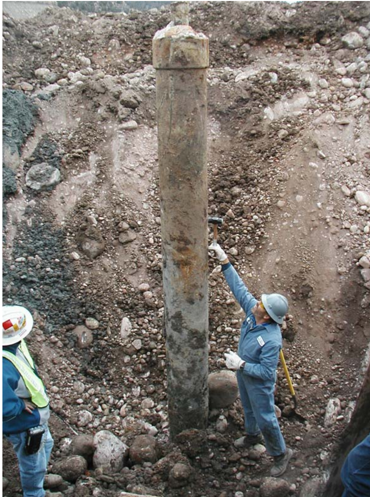
Photograph 4: Inspection of conductor pipe with mallet, view southeast.
