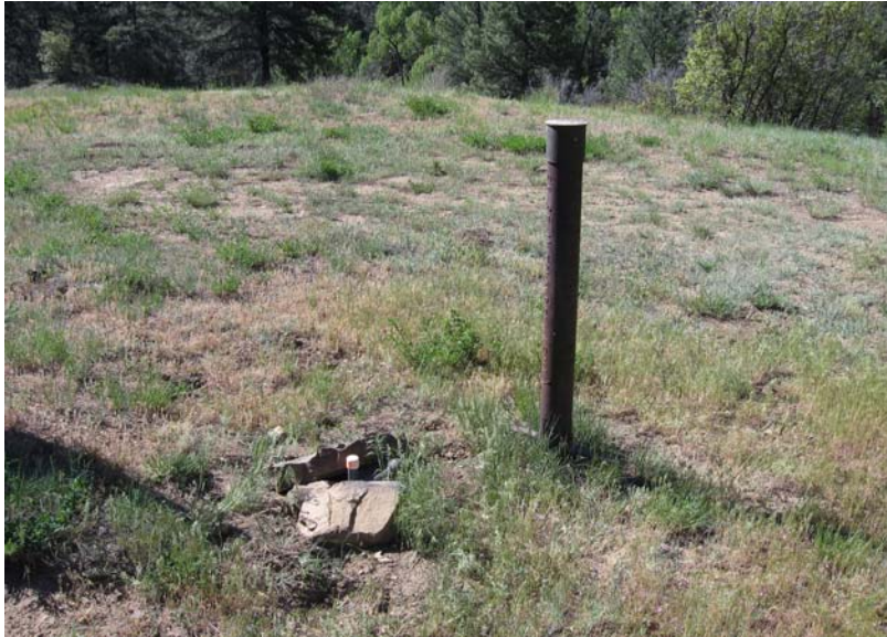
Schomburg #1 abandoned well marker and permanent gas monitoring probe.
