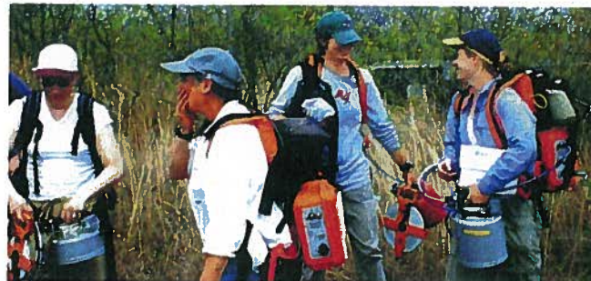
a group of researchers during a flux mapping fieldwork, using the WS-LI820 flux meter Courtesy of United States Geological Survey
