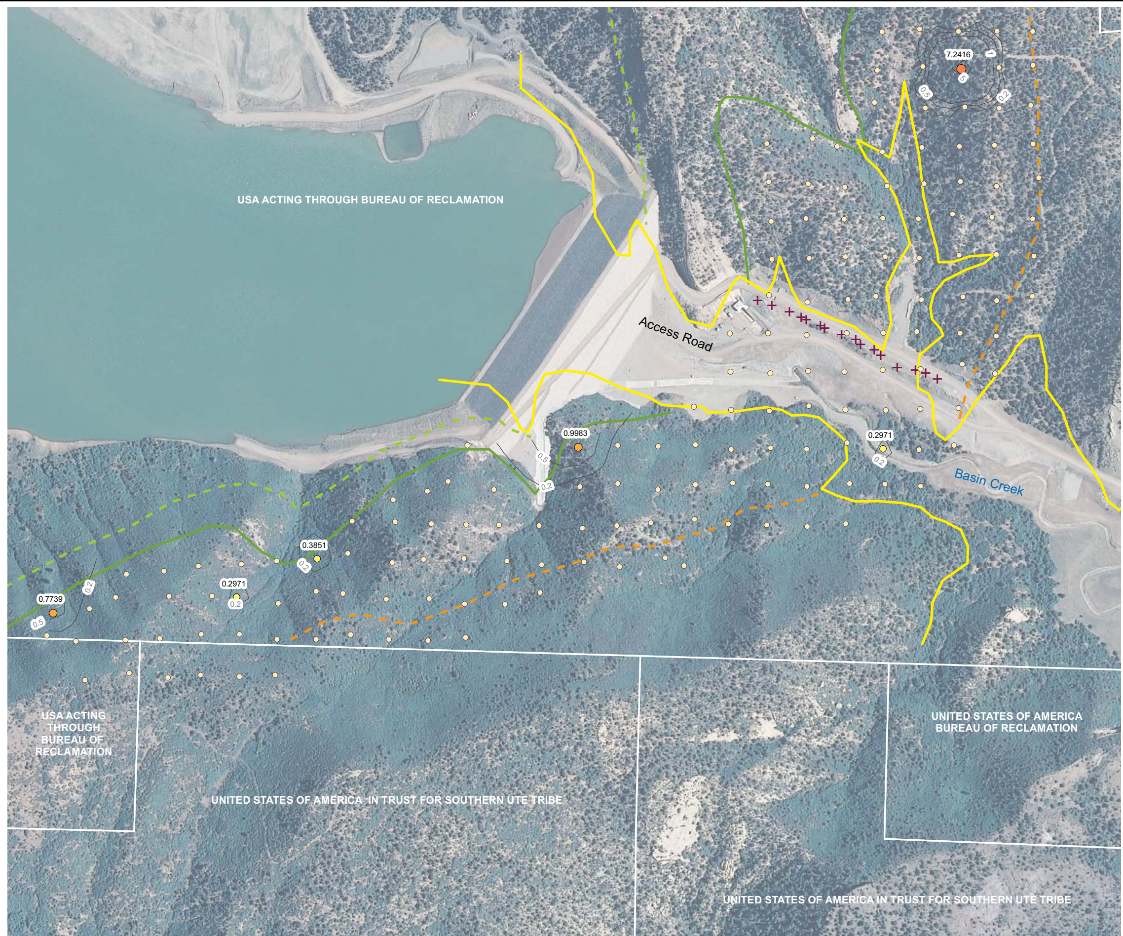
FIGURE 2 METHANE FLUX CONTOURS BASIN CREEK 2010 FRUITLAND OUTCROP MONITORING LA PLATA COUNTY, COLORADO THE GROUP
