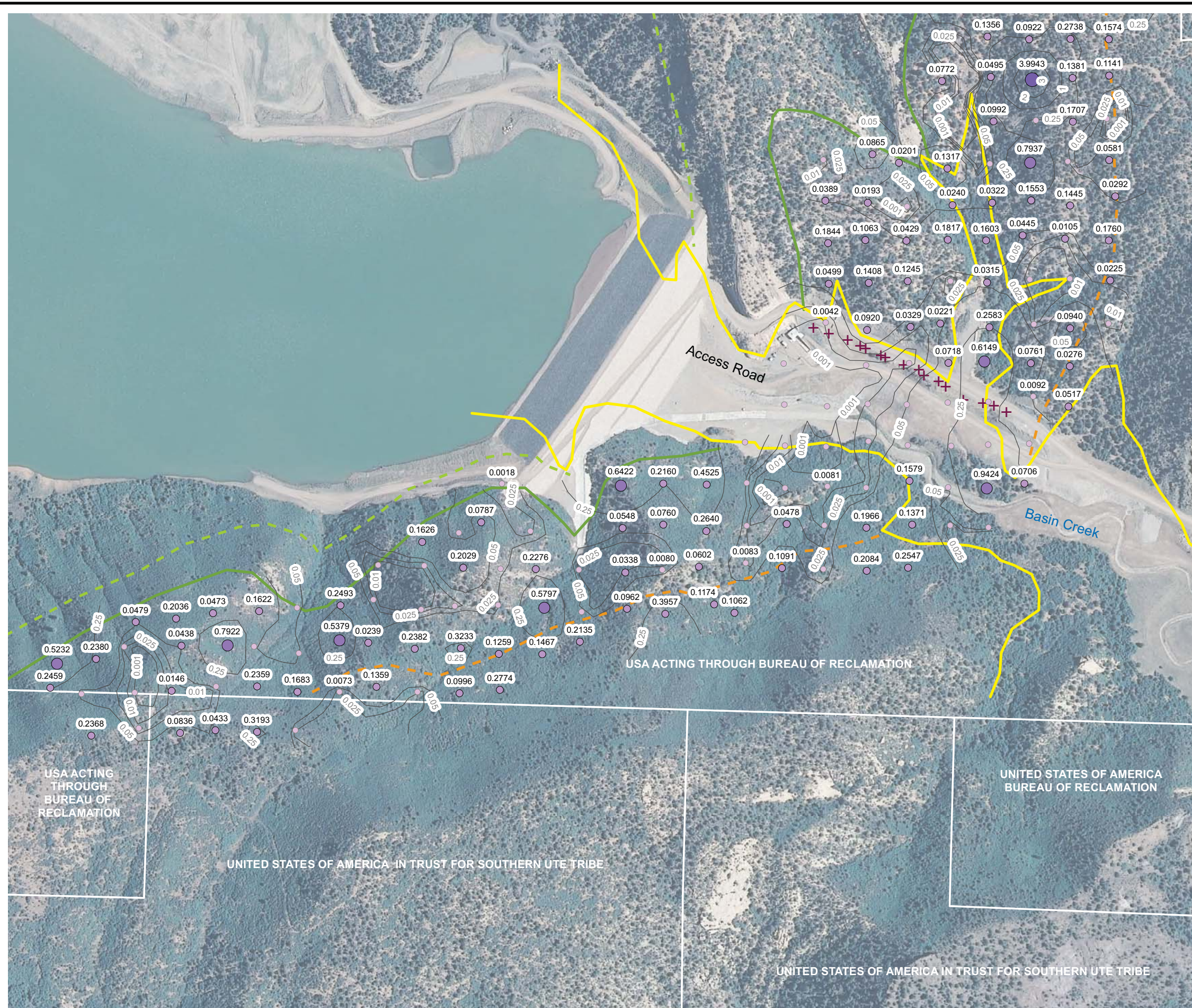
FIGURE 3 CARBON DIOXIDE FLUX CONTOURS BASIN CREEK 2010 FRUITLAND OUTCROP MONITORING LA PLATA COUNTY, COLORADO THE GROUP
