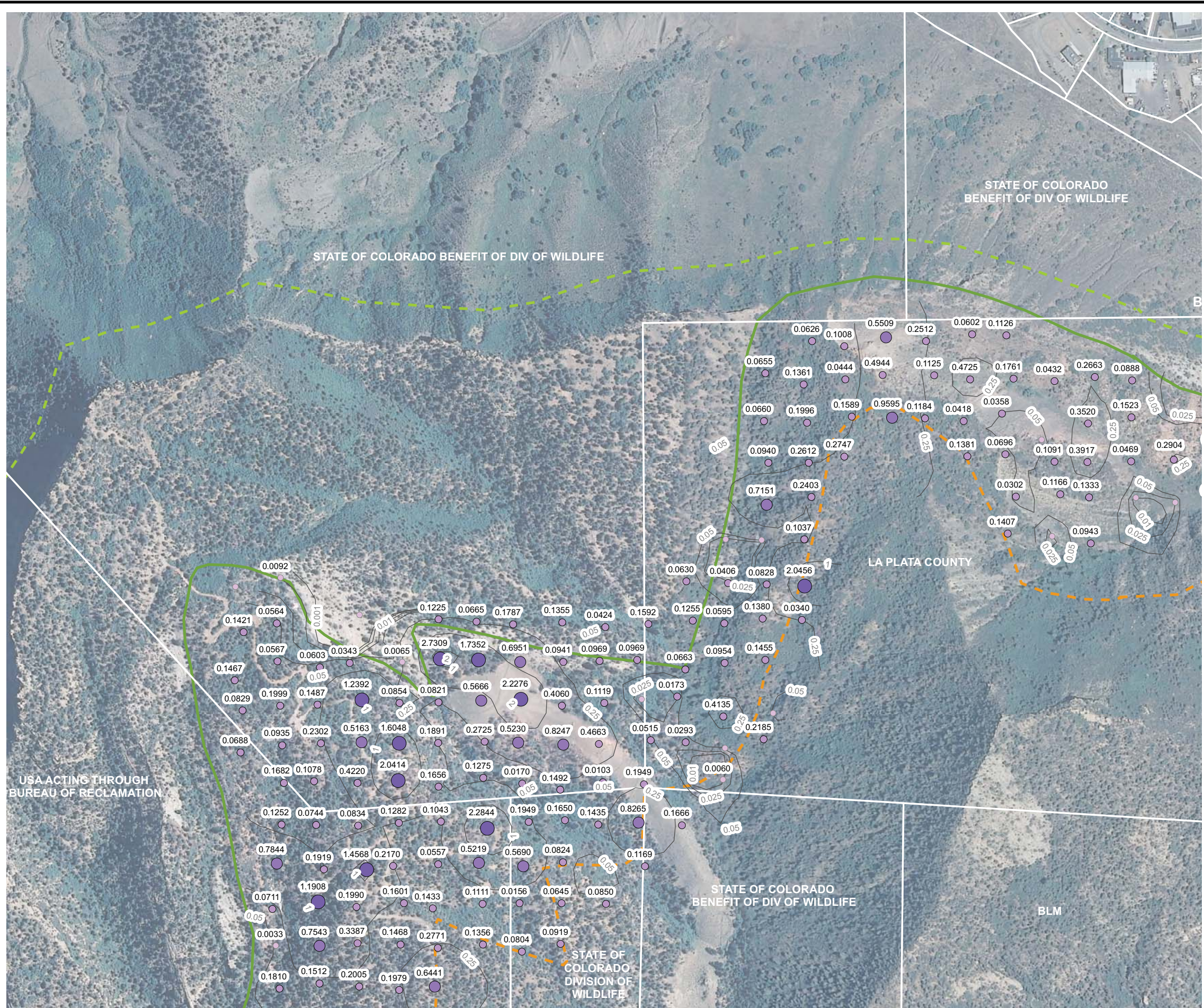
FIGURE 5 CARBON DIOXIDE FLUX CONTOURS BASIN CREEK NORTH 2010 FRUITLAND OUTCROP MONITORING LA PLATA COUNTY, COLORADO THE GROUP
