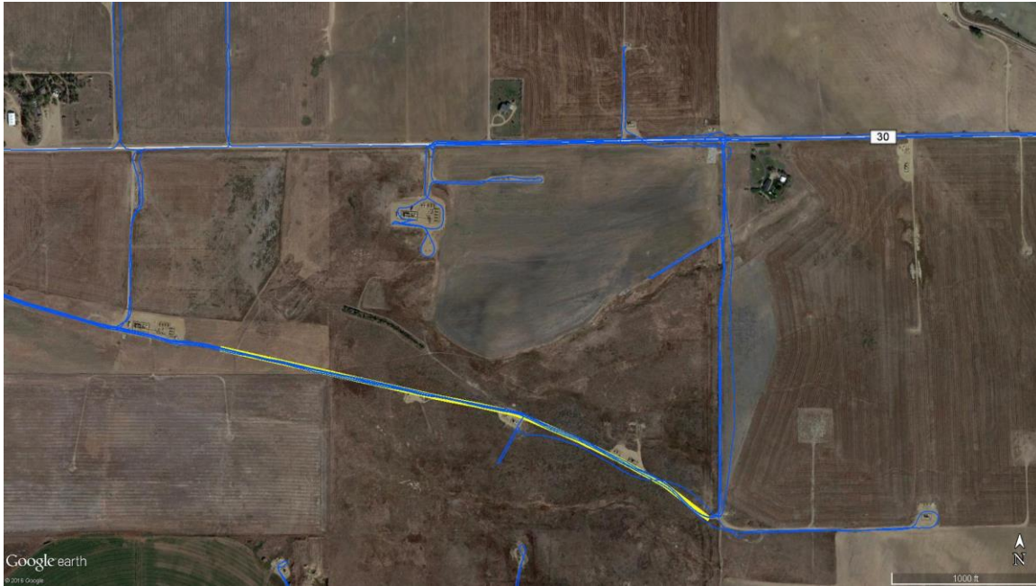
Figure 4. Map of Potential Seep A. The blue line is the track of the survey vehicle and the yellow line is the area where an elevated methane concentration was observed.
