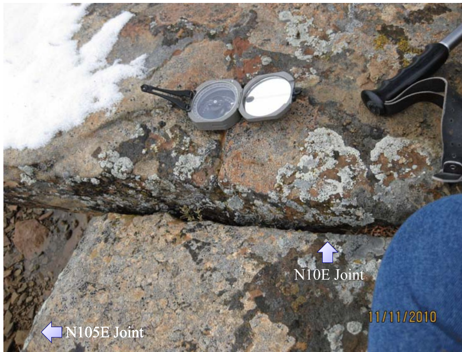
Photograph 4 - P3 Well Pad Outcrop View of the N105E joint set truncating against the N10E joint set.
