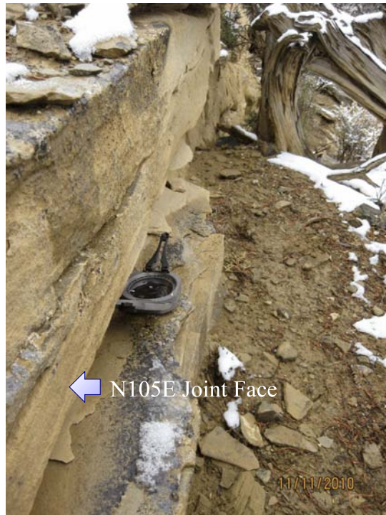
Photograph 2 - P3 Well Pad Outcrop View to the east of the primary vertical joint set; oriented N105E.
