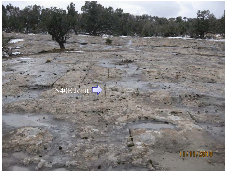
Photograph 8 - Bracken Outcrop View to the southwest of the surface expression of the N40E joint set.
