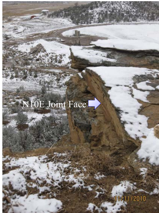
Photograph 3 - P3 Well Pad Outcrop View to the south of the secondary vertical joint set; oriented N10E.
