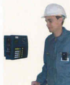
Technician using the hands-free capability of the DMC 2000S with LDM 2000 reader.
