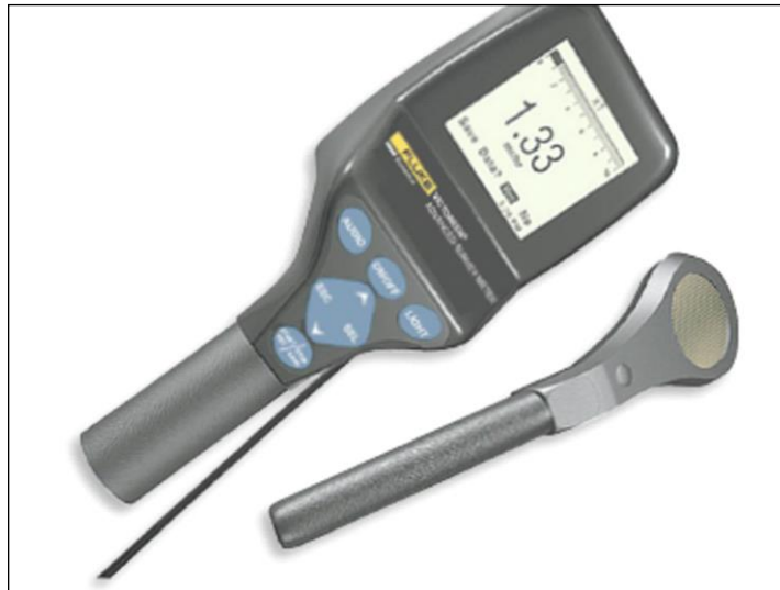
Fluke ASM-990 with 489-110D Geiger-Mueller Pancake Probe
