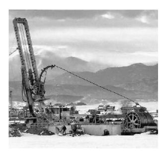
Anadarko Petroleum began using a coiled tube rig in November in the Wattenberg oil and gas field in eastern Colorado. The newer rigs are smaller and more portable than standard rigs. (Special)
