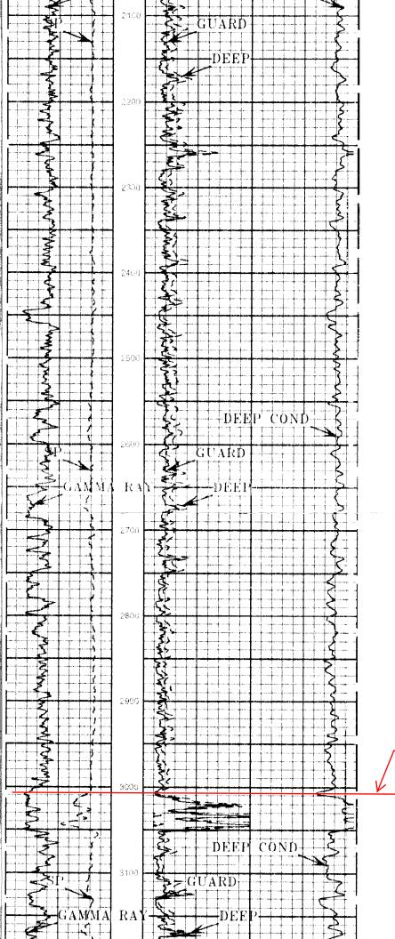
COGCC pick for Lower Wasatch top (cement required 200'/500' above this point, effective 04-18-2016)
